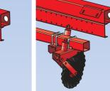
FLOATING COULTERS TO BAR Used when soil surfaces have logs
