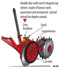
A good no-till farming is achieved by placing the seed at the desired and constant depth, with close soil-seed contact.
