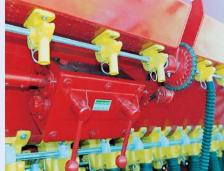
The alfalfa distribution system is of maximum precision. Plastic helicoidal distributors driven by gearbox offer accuracy in time and minimum quantities from 1kg per hectare are possible. Desired depth is achieved by means of continuous adjustment, controlled by the delivery tube in the seeding unit.
